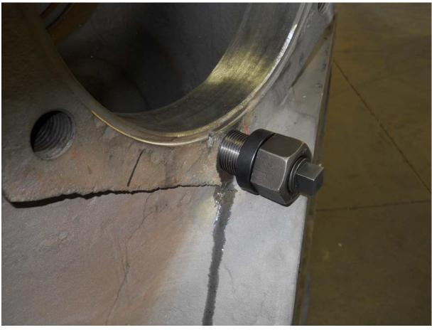
**Completion of Stitching and Insert Repair**
