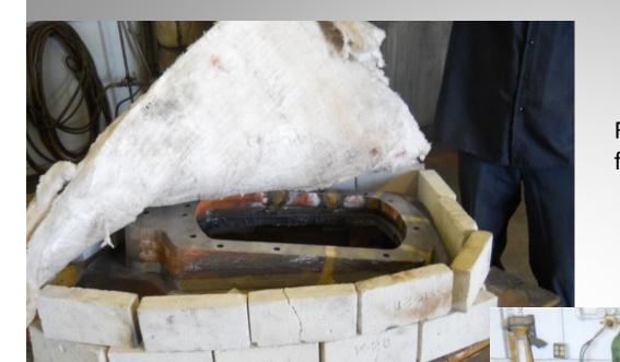
Flange set up in oven and ready to be furnace brazed
