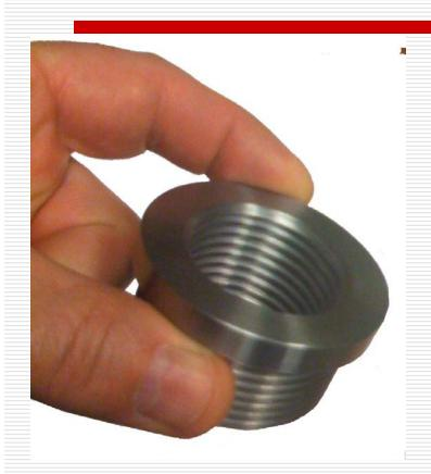
Full-Torque thread repair inserts are made with our patented Spiralhook threads on the outside and standard threads on the inside. The shoulder seats into a special machined spotface that adds to the drawing force when installed.
