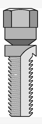
castmaster stitching pins have the unique ability to draw the sides of a crack together when tightened into the drilled, Spotfaced and tapped hole.
