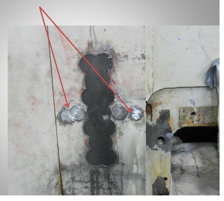
Receiving pattern for the L30 lock on the side frame of the press.
