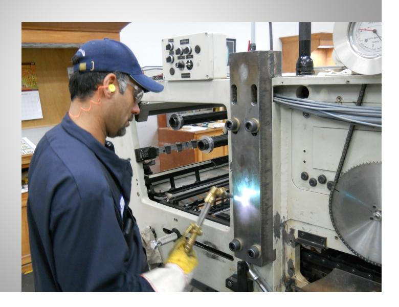
An additional bracket was mounted on the opposite side of the press to strengthen it as well.
