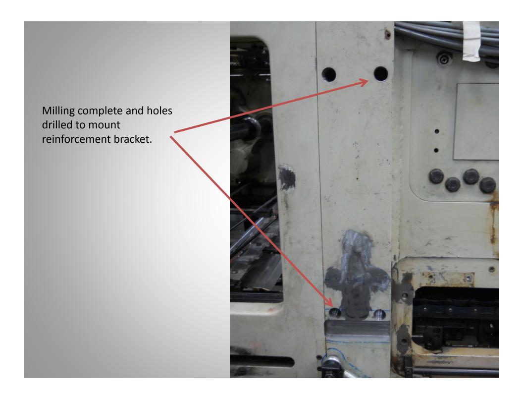
The bracket was bolted over the stitching repair. When heated the bracket grew in length and shims were placed under the overhang at the top of the bracket so as it cools the bracket is under tension to add strength to the area and make it stronger than new.
