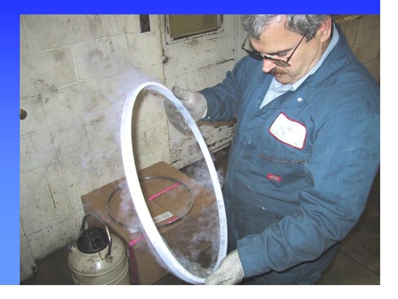
The repair sleeve is installed in the bore and expands with a .005" press fit. The top of the insert registers flush to .002" above the fire deck surface
