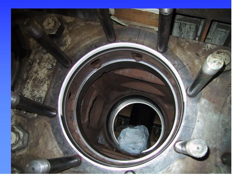
The sleeve produces a new gasket seal surface that can be replaced in the future if necessary without need of machine work.
