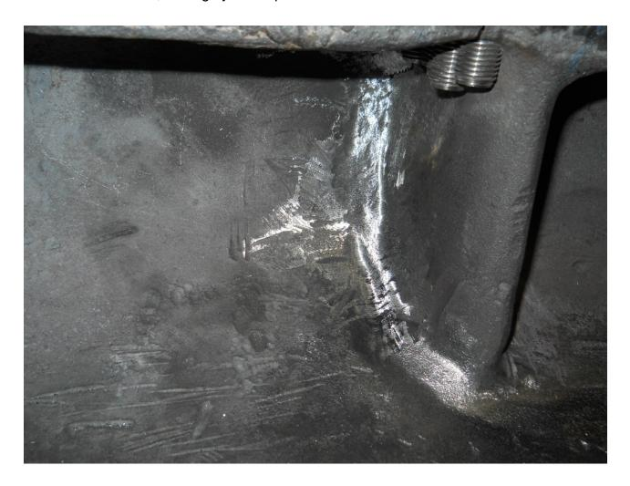
Completed crack repair for 1H and 1J:
