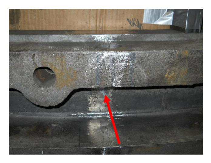
1FShows the thickness of the lower flange (2.75" thick)
