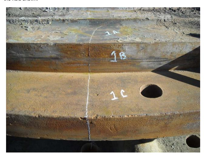
Metal stitched 1C, 5.125" long by 2.5" deep, using C4C stitching pins; and 2.5" long by 0.5" deep using C2.5A stitching pins, on outside of outer bolt hole flange.
