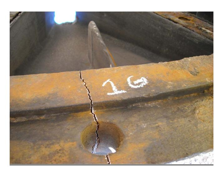
Metal stitched 1G crack, 2.75" long by 3" deep, using C4C stitching pins.
