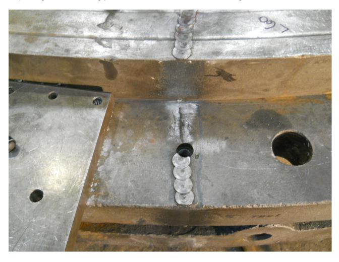
Installed (1) L60S lock, (4) L60B locks, (1) L40S lock and (4) L40B locks in 1C. (Retained locks with (4) L6A pins).
