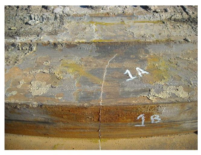
Metal stitched 1A: 4.5" long by 2" deep, using C4B stitching pins and 2" long by 1" deep using C3B stitching pins.
