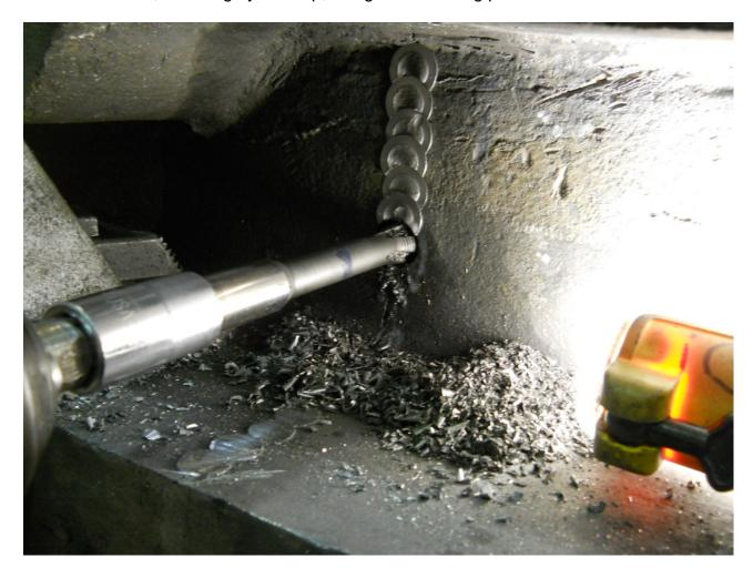
Installed (2) surface L40S locks and (6) L40B bottom locks in 1D. (Retained locks with (2) L6A pins).
