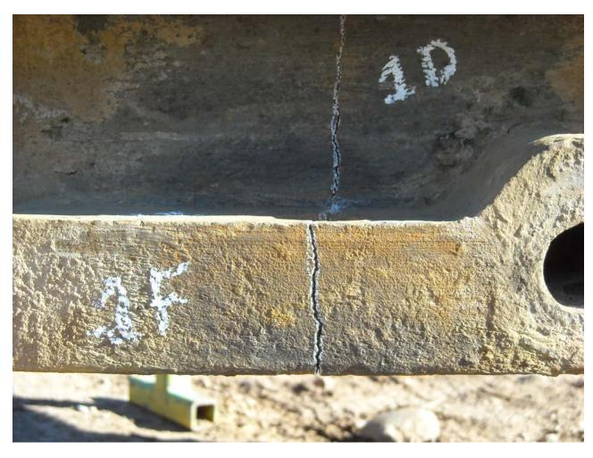
Metal stitched 1F crack, 2.75" long by 0.5" deep, using C2.5A stitching pins.
