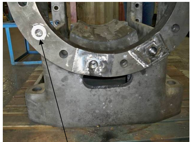
Additional inserts were installed to repair other damaged stud holes
