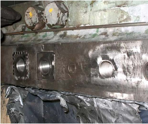
The same concept was used to fill in additional pulled out stud holes
