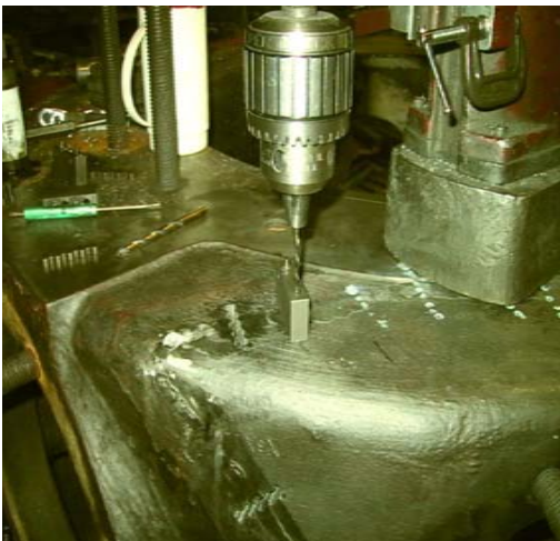
Lock hole patterns are drilled across the joint to accept L20 Locks for added strength
