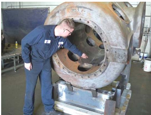
A 36 inch long, \frac{3}{4} inch groove was cut into the liner bore
