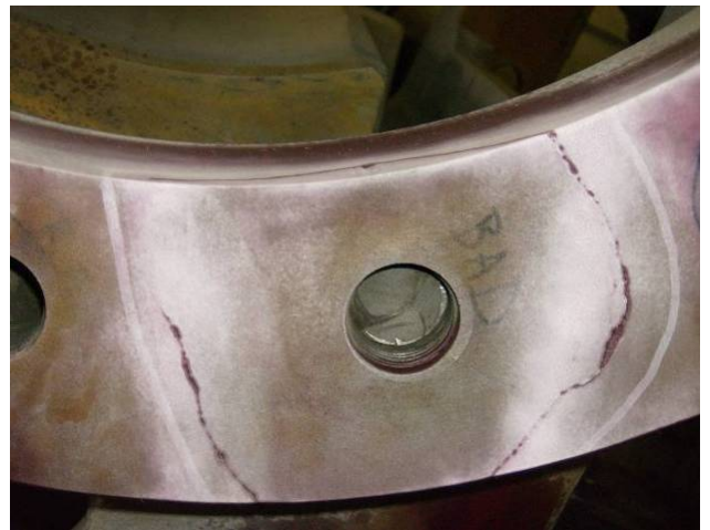
The area outlined by the cracks had to be milled out to receive a steel patch
