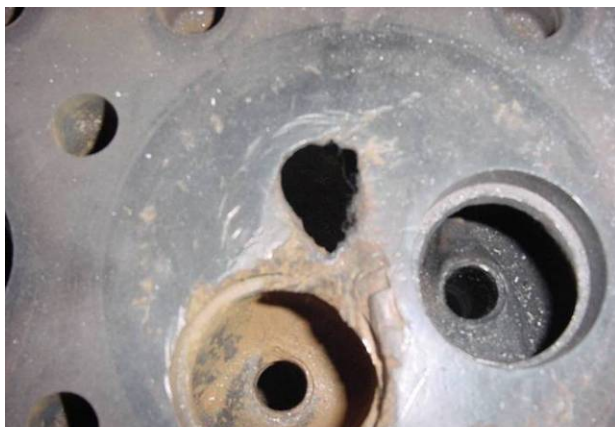
Damaged cylinder head can be repaired by cast iron fusion welding
