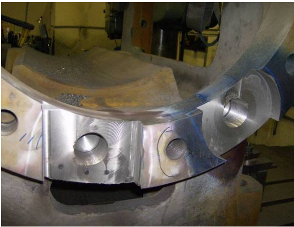
The broken out areas were milled out to accept the new steel plates and tapped to accept the blind Full-Torque thread inserts
