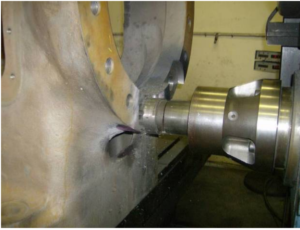
The pulled areas were milled out to receive the patches
