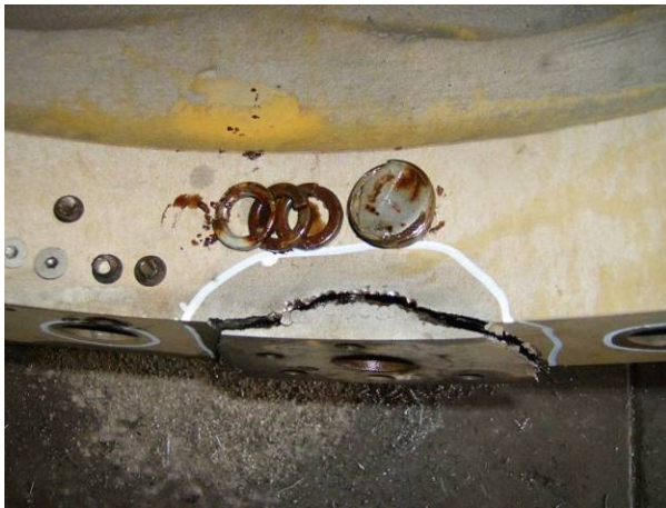
Several stud holes were pulled out when the studs broke about 1 inch below the surface
