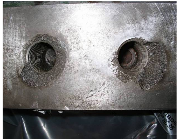
A compressor frame also suffered from pulled bolt holes and was repaired on-site with the same process
