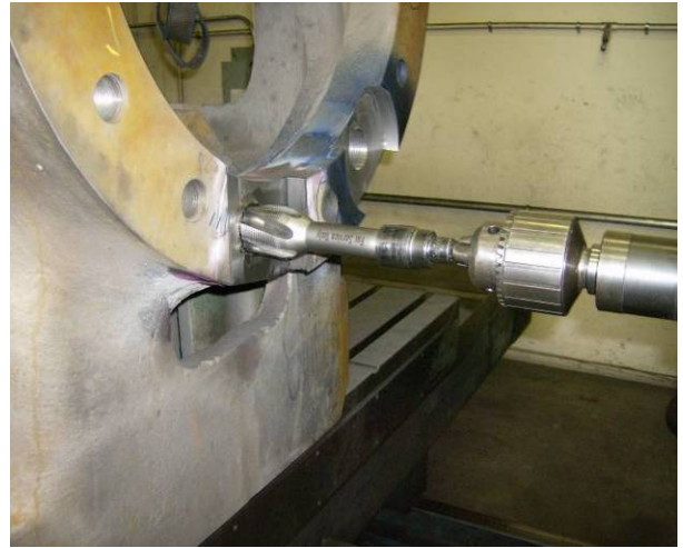
The original holes were drilled and tapped with a special FT tap
