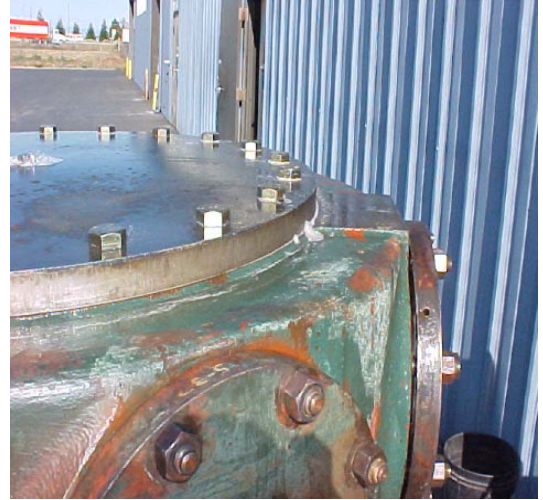
The cylinder was hydro-tested to 420 PSI to validate the integrity of the repair
