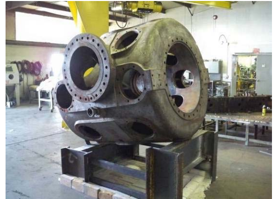
Compressor cylinder damaged trying to remove the liner with an air arc
