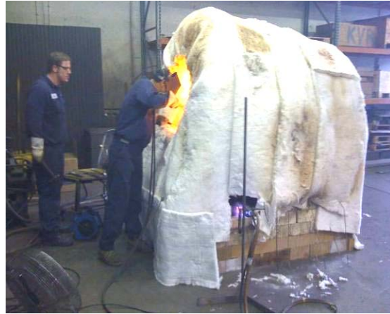
Brazing the upper half of the groove
