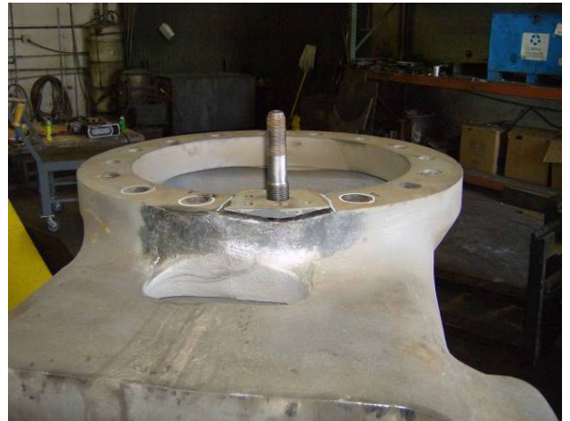
A previous Metalock repair attempt failed and allowed the sections to pull completely out
