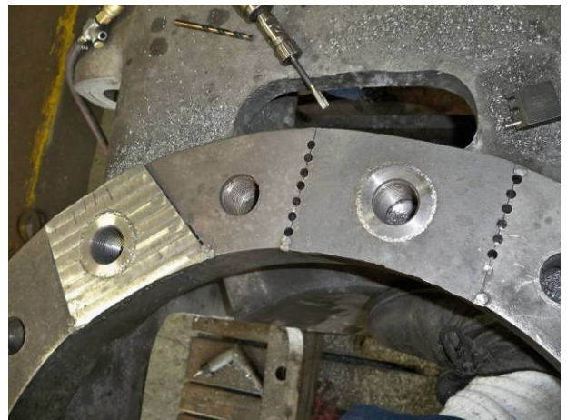
New sections of steel plate fit in and locked in place with FT thread inserts, the joint lines were stitched for strength and high pressure seal
