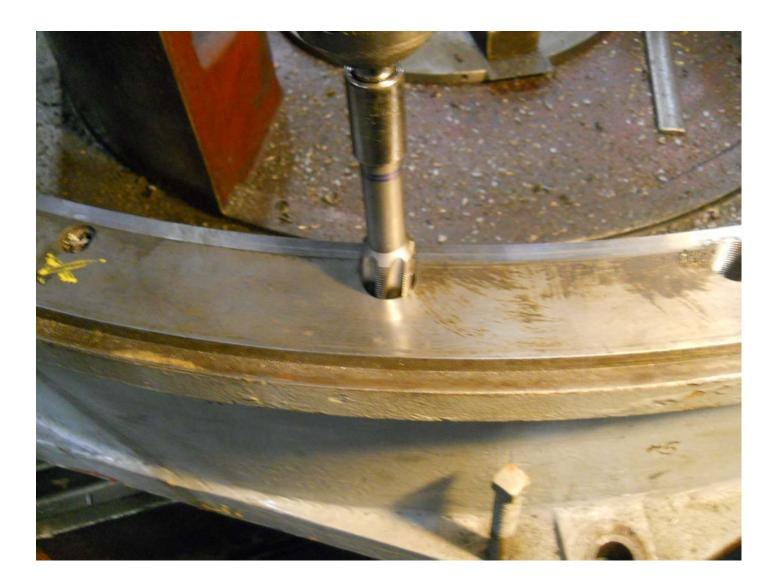
5. Installing the new insert flush with machine surface.
