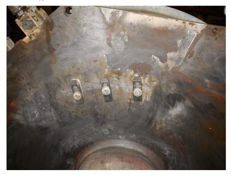
12. The repair was covered with Titanium putty for extra protection.
