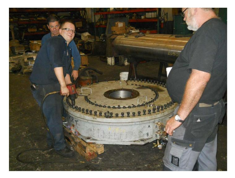
11. Leak was found in a prior repair. Extra stitching pins were installed and
