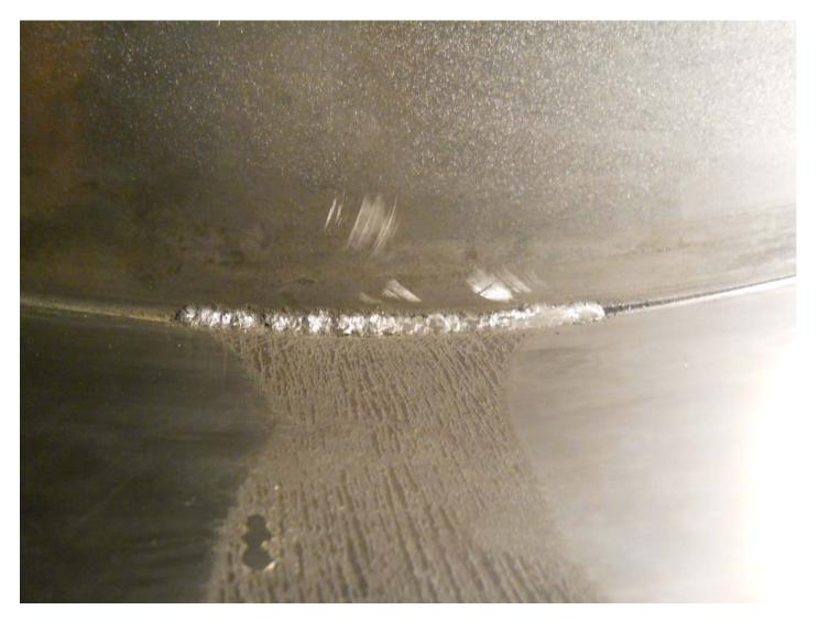
10. Steering pod was pressure tested to check for any leaks. No leaks were found.
