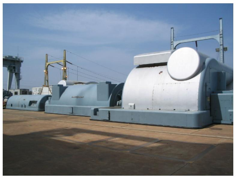
The upper shell was moved to the ground and blocked up.
