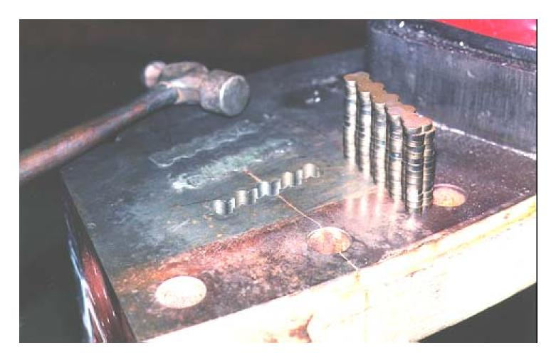
GE Gas turbine shell repaired in 1992 for Sicamore Co-Gen Near Bakersfield California. The unit is still in use. The crack was through the outer bolt flange and was approximately 800mm long and 75mm thick.
