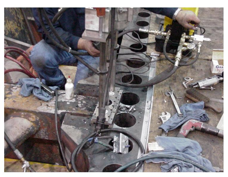
The hole pattern for the L60 locks has been drilled across the crack. The locks were installed 125mm deep.
