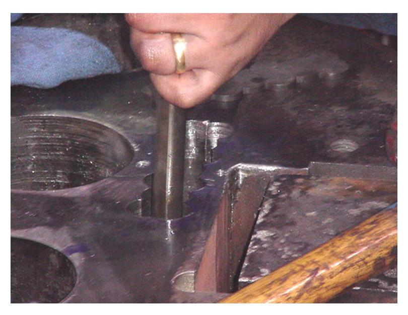
The locks are installed and ready to be machined flush
