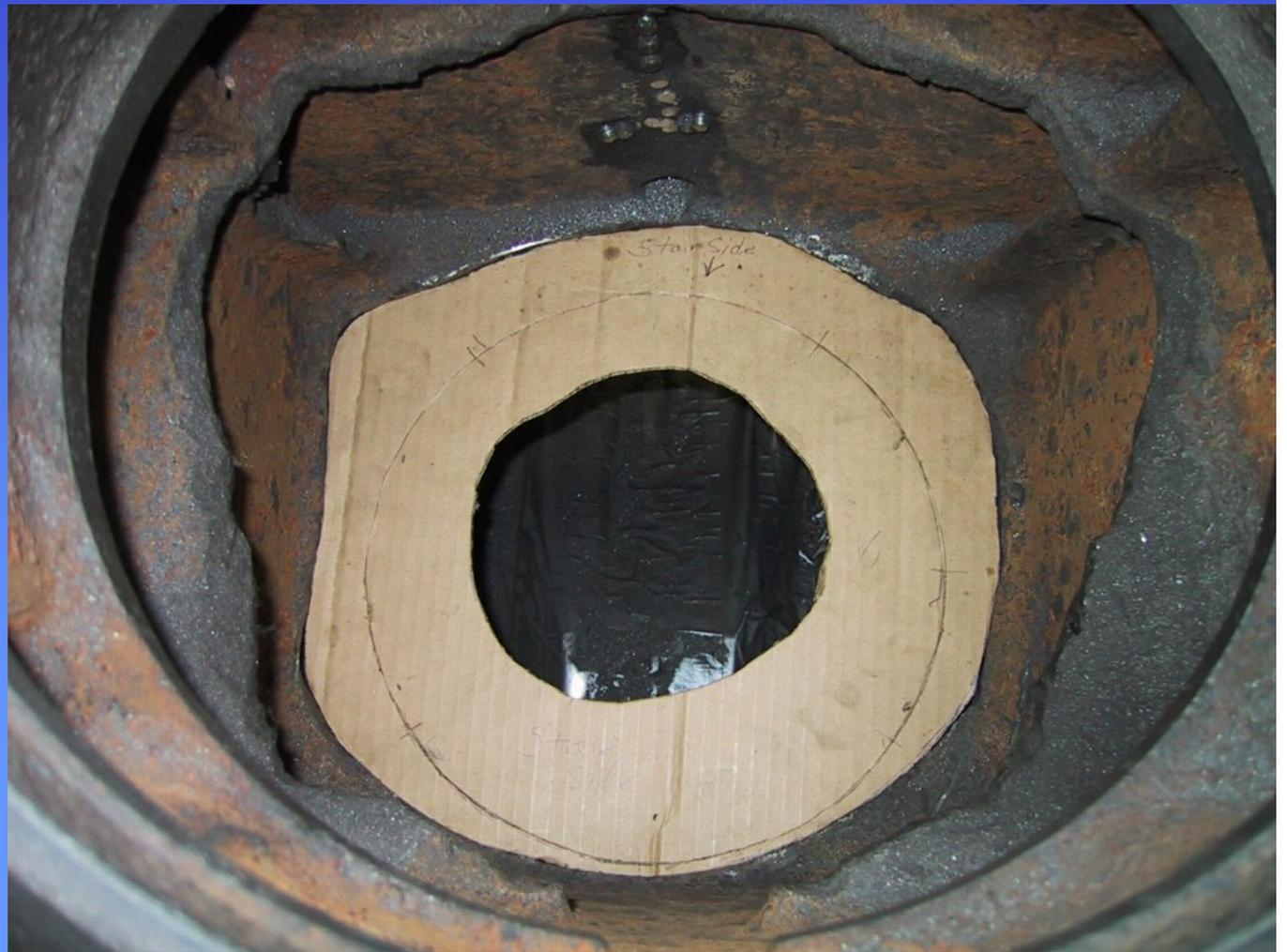
The approximate center of the bore was cut into the template
