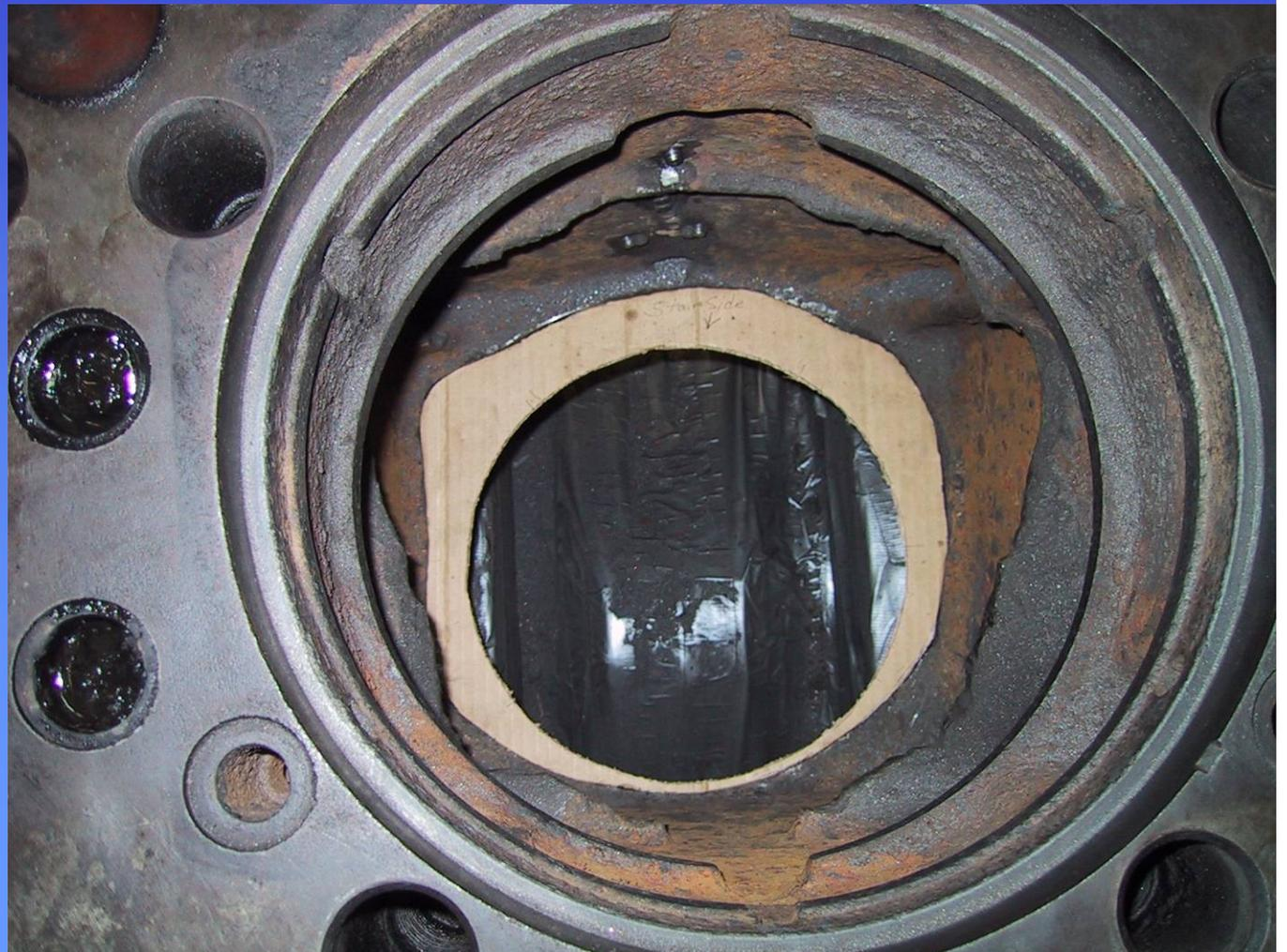
A new section was cast to cut the replacement piece from
