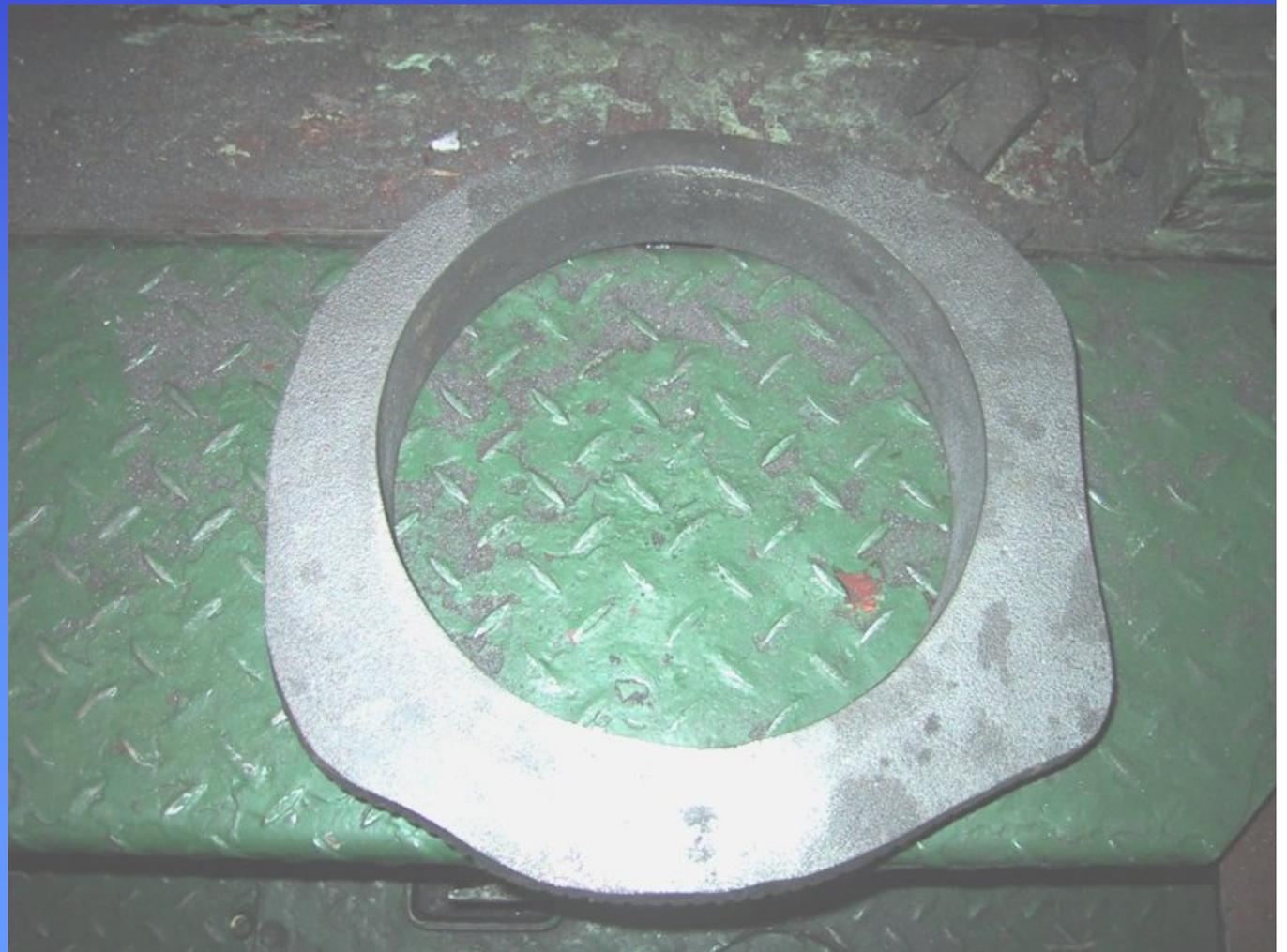
A few stitching pins were installed into the joint to secure the new piece
