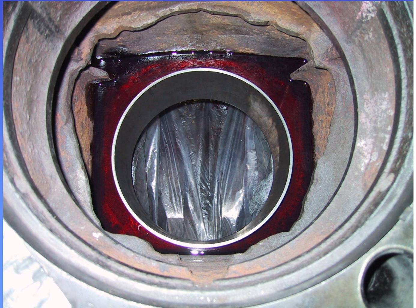
The new liner and piston are installed
