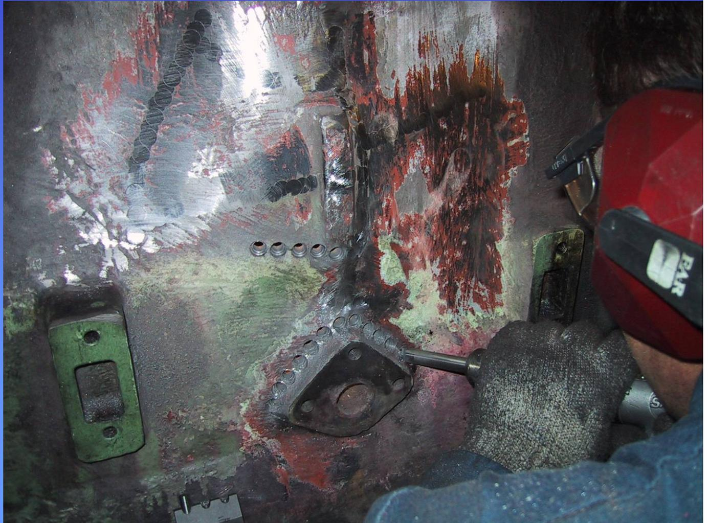
After the CASTMASTER stitching pins are installed, lock hole patterns are drilled across the repairs.
