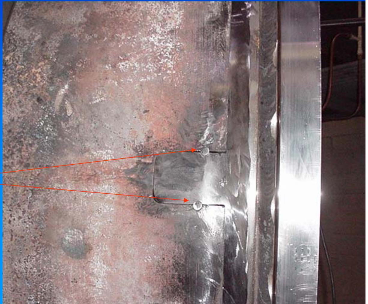
Stitching around the locking-lugs adds strength to the joint
