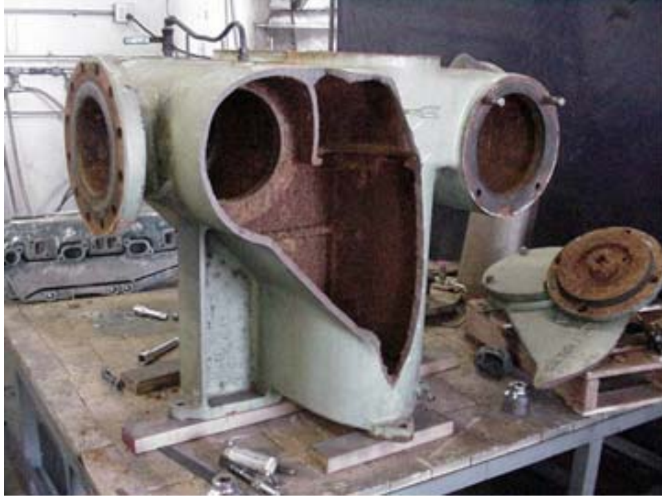
Over pressurization blew the side out of this casting.
