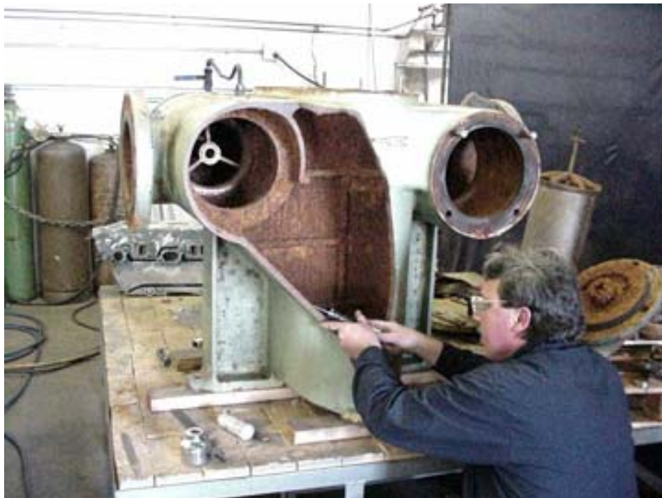
Casting is prepared for high temperature brazing.
