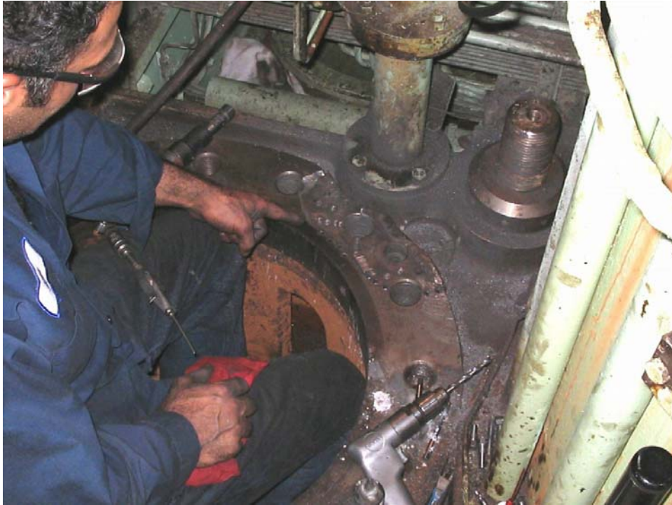
Stitching continues to reattach the broken out pieces
