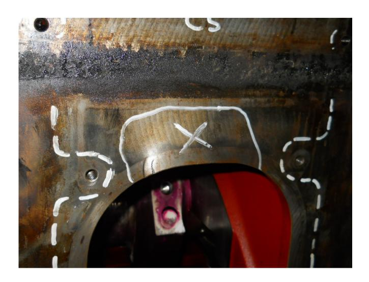
The damaged area has been cut out to accept new casting.
