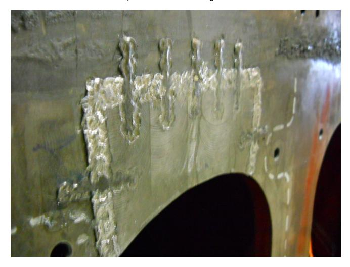
Set up and machine inspection window seal surface at exhaust side and cam box side.
