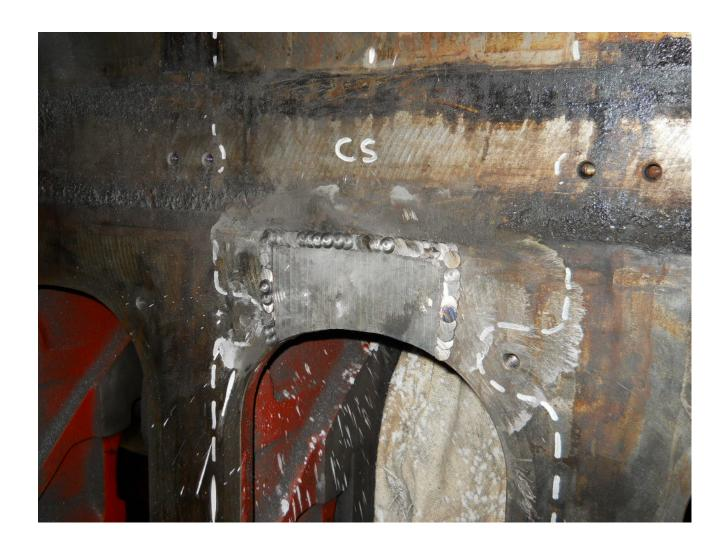
L20 locks installed around the repair for additional strength.
