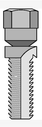
castmaster stitching pins have the unique ability to draw the sides of a crack together when tightened into the drilled, Spotfaced and tapped hole.
