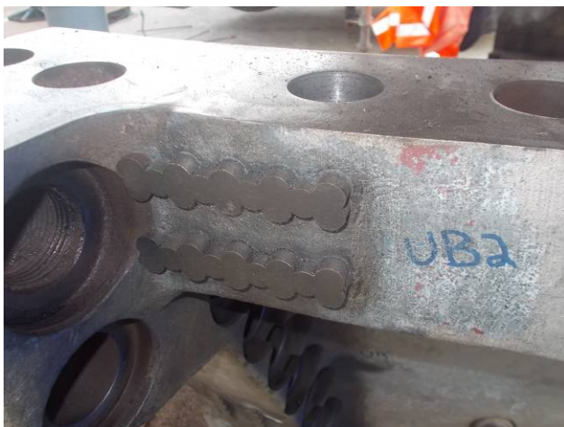
Stitching, locks, and insert complete
