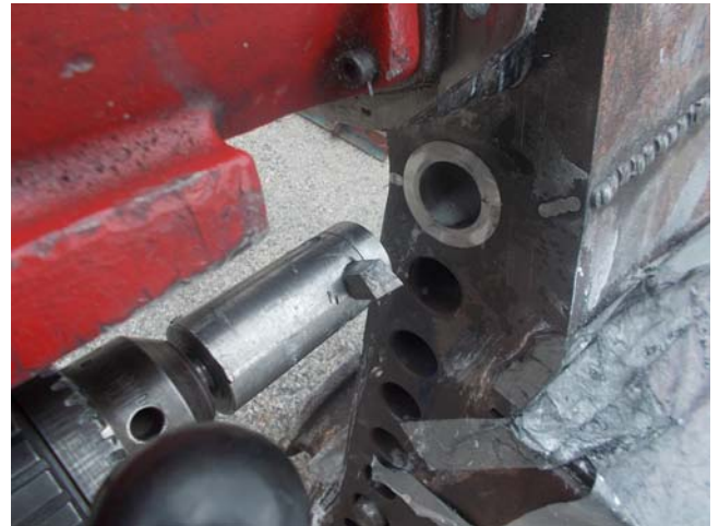
Facing off the insert to match part
