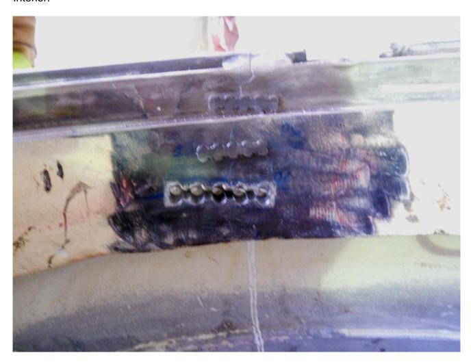
Metal stitch remaining cracks with C3 high-strength Castmaster pins.
