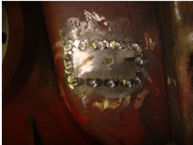
#7: Metal stitched in second row of pins with over lapping fashion.
