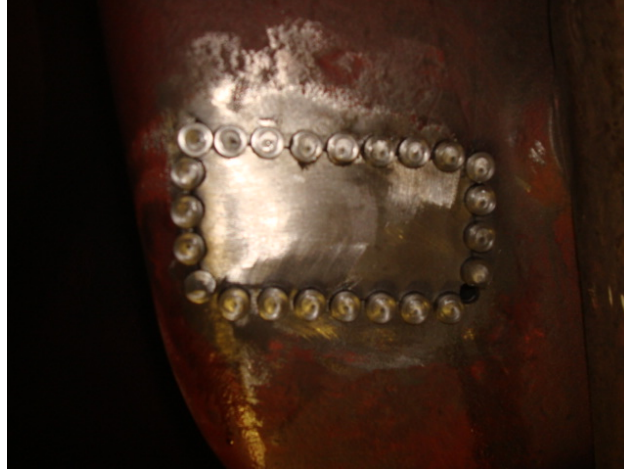
#6: Metal stitched in first row of C2.5 pins.
