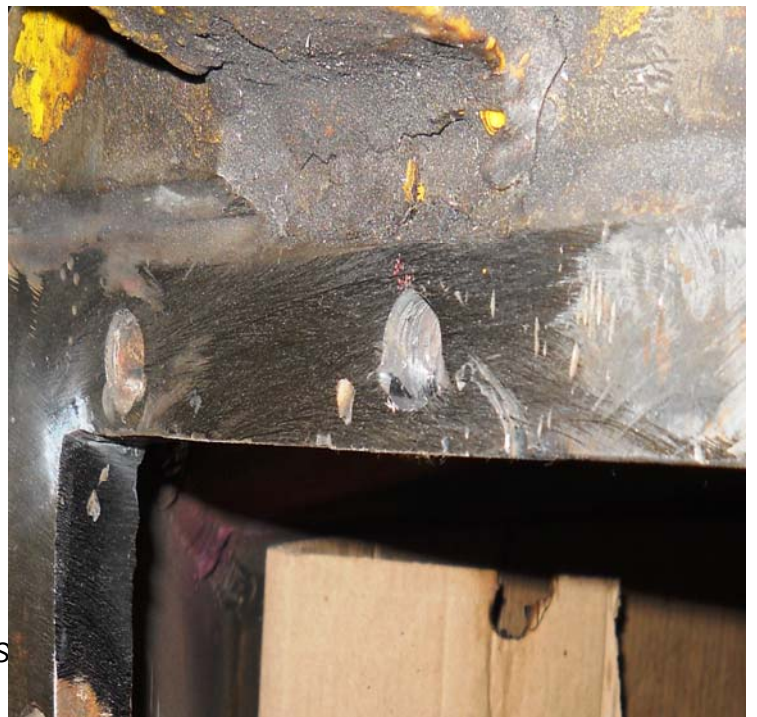
Two broken stud holes welded
