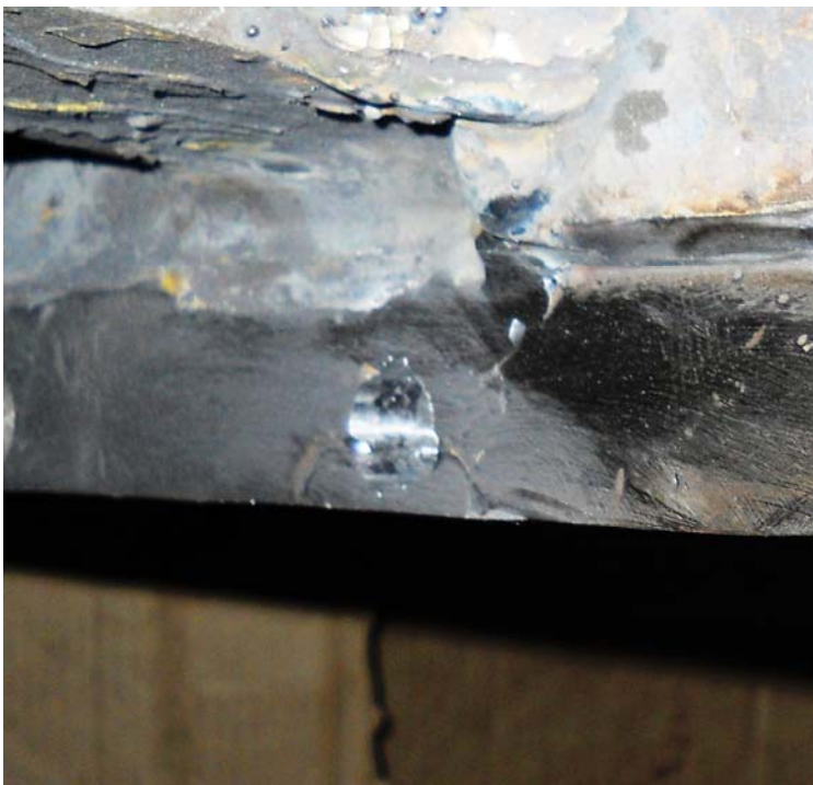
Two broken stud holes welded
