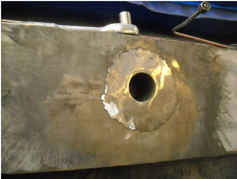
Second row of stitching pins Installed and ground close for final machining.
