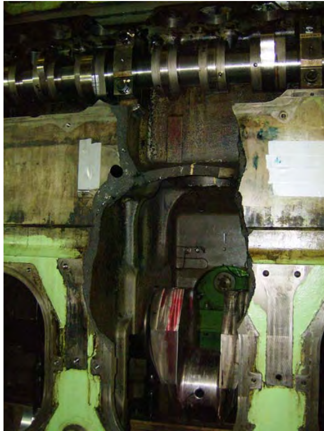
Large hole on sidewall of engine block
