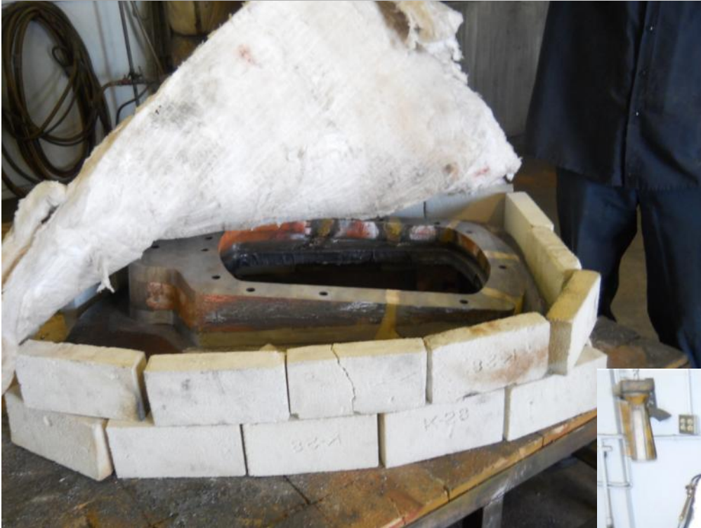
Flange set up in oven and ready to be furnace brazed
